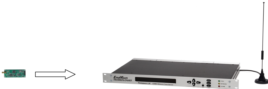
Figure 2. PTP Grandmaster Clock
