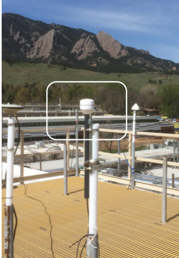
Figure 1: Meridian II Precision GPS antenna attached to antenna mounts on the fiber glass platform atop NIST, Boulder, Bldg. 1 roof.
