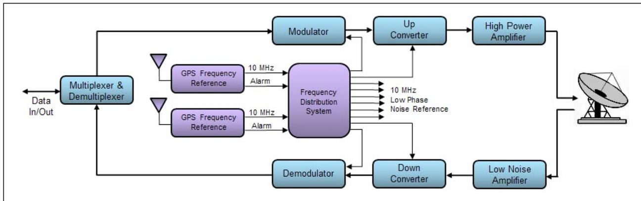
Figure 1. Dual GPS Frequency Reference and Distribution System
